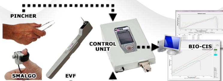
Export data from the Smalgo, Electronic Van Frey & Pincher to Microsoft Excel
